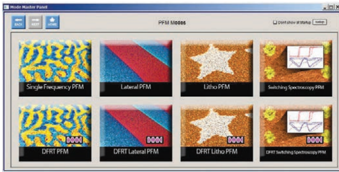
Figure 20: MFP-3D Piezo Force Module software menu allows easy point and click navigation.
