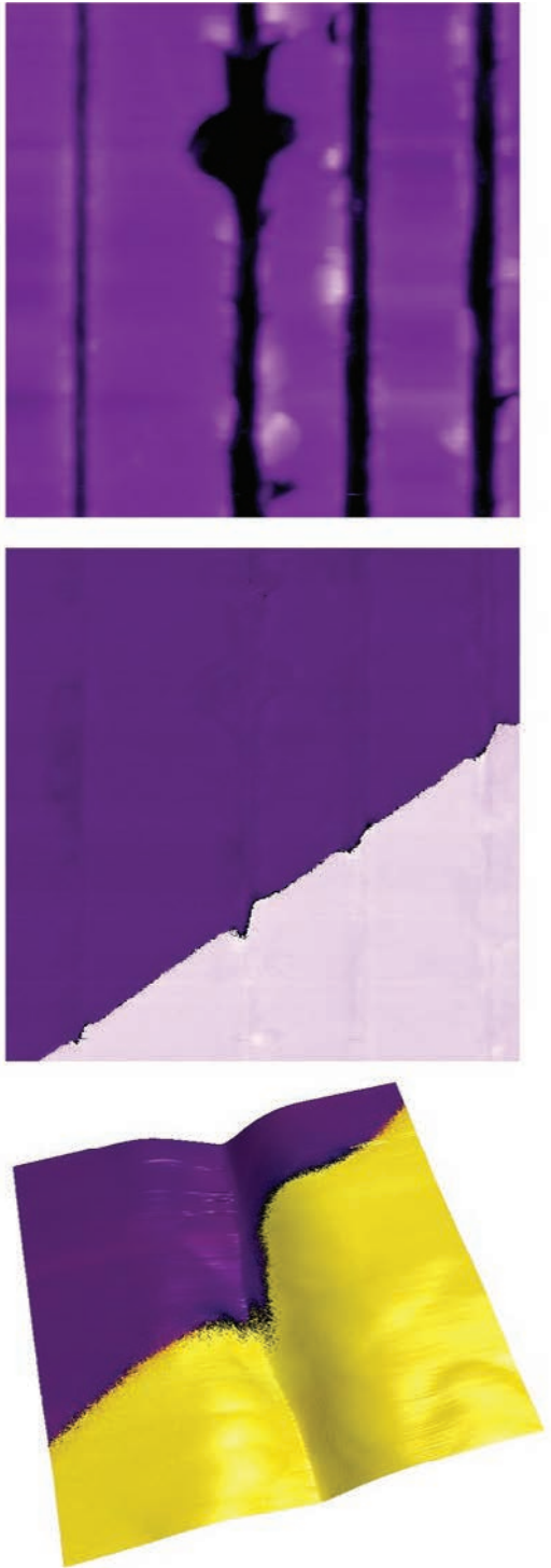
Figure 32: Surface topography of PPLN after it has been purposefully scratched with different loading forces using the NanoIndenter, 10 \mu\text{m} scan (top and middle images). 1 \mu\text{m} scan (bottom).
