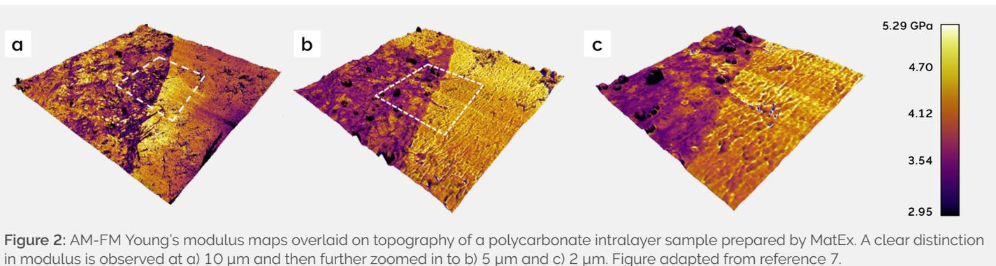
**Figure 2:** AM-FM Young's modulus maps overlaid on topography of a polycarbonate intralayer sample prepared by MatEx. A clear distinction in modulus is observed at a) 10 µm and then further zoomed in to b) 5 µm and c) 2 µm. Figure adapted from reference 7.
