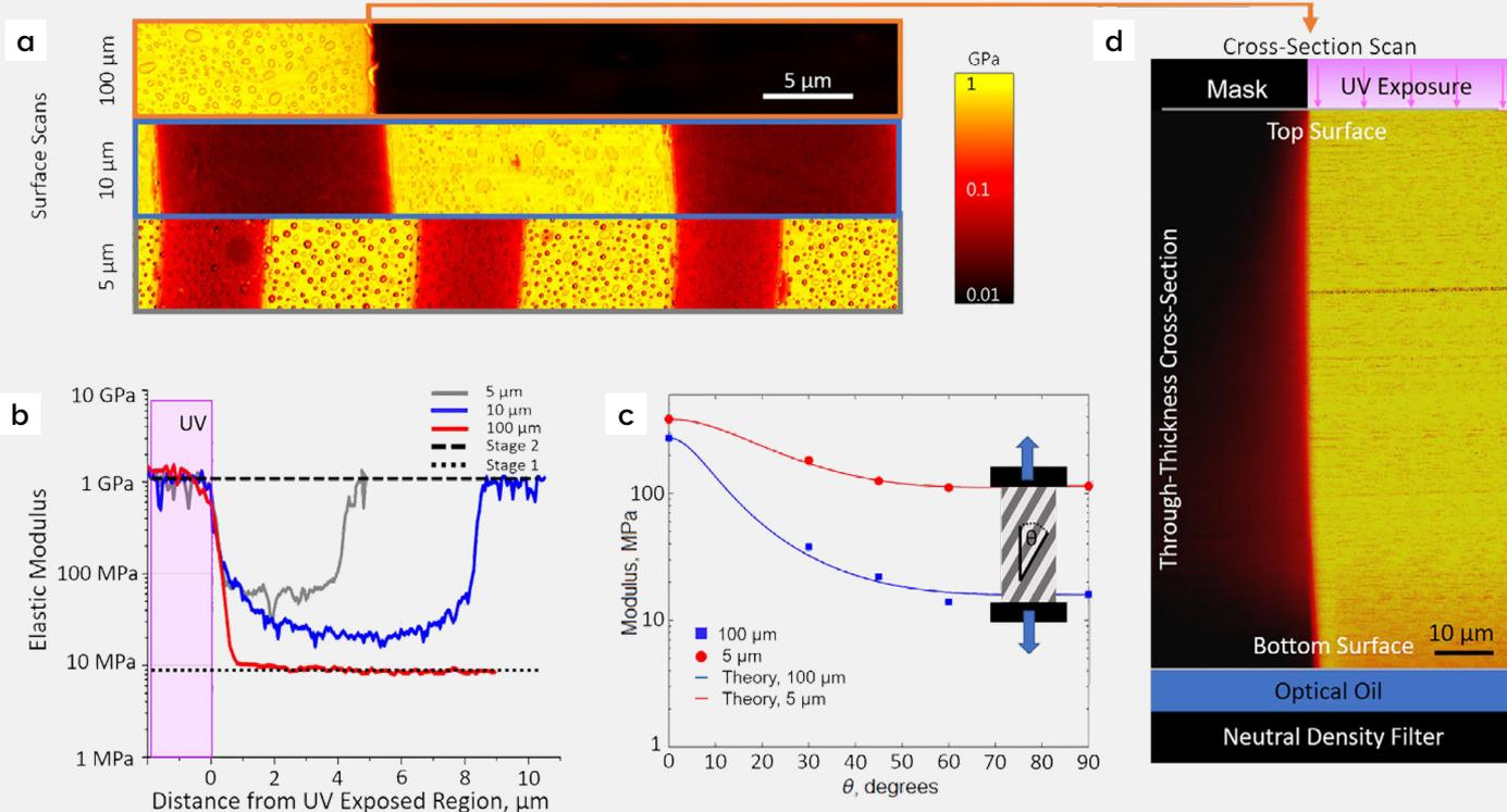
**Figure 3:** a) FFM Young's modulus maps of TSRPs with different sized photomasks applied. b) Line section profiles across interfaces of masked and unmasked areas. c) Modulus measurements at different loading angles from dynamic mechanical analysis (DMA), showing anisotropy d) FFM Young's modulus map of a cross section of a TSRP layer showing good uniformity. Figure adapted from reference 11.
