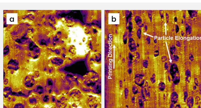
Figure 1: Topography images of ABS samples prepared by a) injection molding and b) Fused deposition modeling AM. Elongation and alignment of the butadiene particles are observed in the sample prepared by AM. Figure adapted from reference 2.
