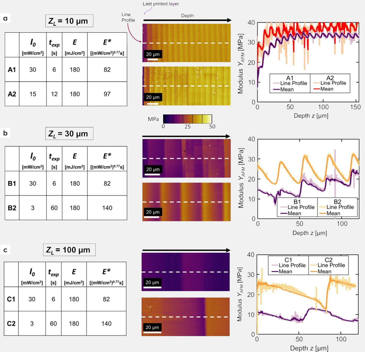
Figure 4: FFM Young's modulus maps of through-thickness 3D-printed structures, different exposure intensities ( $I_0$ ) and time ( $t_{exp}$ ) for layer thicknesses ( $Z_L$ ) of a) 10  $\mu\text{m}$ , b) 30  $\mu\text{m}$  and c) 100  $\mu\text{m}$ . Thin layer thicknesses produced layers of material with step changes in modulus whereas thicker layers produce a gradient. A lower  $I_0$  and longer  $t_{exp}$  leads to an overall higher modulus. Figure adapted from reference 14.
