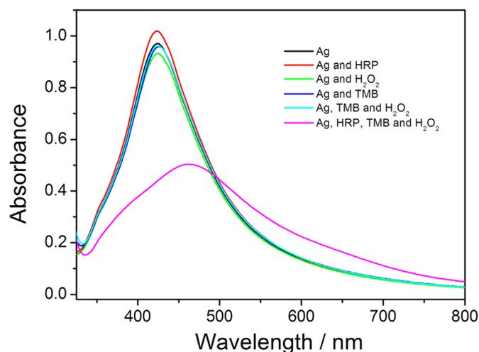
**Fig. 2.** UV–vis absorption spectra of the AgNPs in solution upon addition of TMB,  $\text{H}_2\text{O}_2$ , HRP, and the enzyme reaction product.  $45\ \mu\text{L}$  of AgNPs,  $100\ \mu\text{L}$  of substrate solution, and  $5\ \mu\text{L}$  of HRP (10 ng/mL) were diluted to  $500\ \mu\text{L}$  and the spectra taken after 10 min of incubation.
