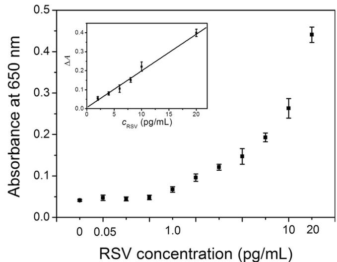
**Fig. 5.** The absorption change at 650 nm versus RSV concentration. Inset shows a linear relationship between the absorbance and the concentration of RSV within the range of 2 to 20 pg/mL (coefficient of determination,  $R=0.994$ ). Error bars indicate standard deviations from three measurements.
