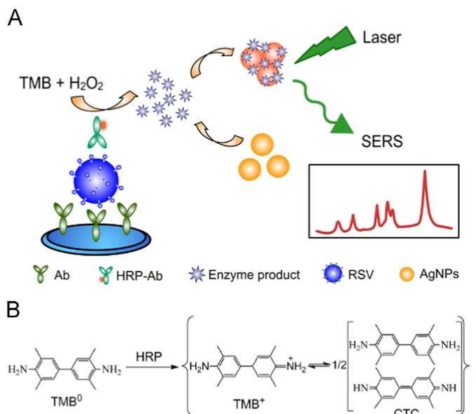
**Scheme 1.** Principle of the SERS-based immunoassay. (A) Sandwich-like immunoassay for RSV sensitive detection using enzyme-catalyzed reaction. (B) Oxidation of TMB by  $\text{H}_2\text{O}_2$  in the presence of HRP.
