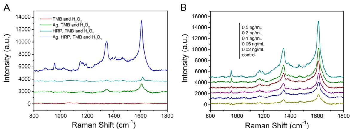
**Fig. 1.** (A) Typical SERS responses obtained in TMB oxidation process. (B) SERS signals in response to HRP at different concentrations: 0, 0.02, 0.05, 0.1, 0.2, and 0.5 ng/mL. The Raman spectra were recorded after 10 min of incubation.
