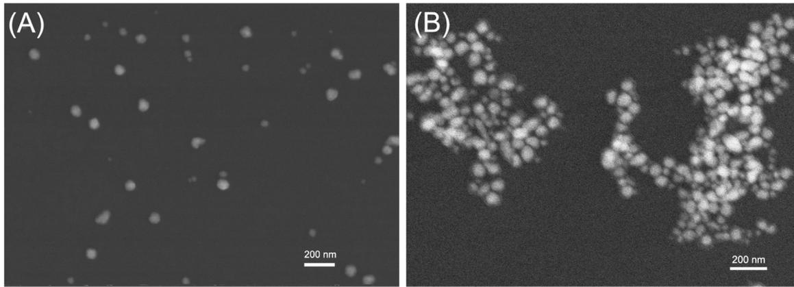
**Fig. 3.** Typical SEM images of AgNPs in the substrate solution (A) and the enzyme reaction product solution (B) after 10 min of incubation.
